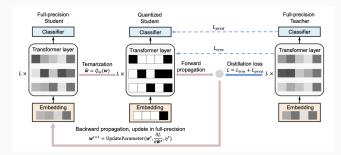
Logits-based loss, the third distillation loss: the loss between teacher model's logits and the student model's logits.
