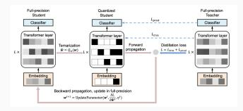
Activation loss, the first distillation loss: knowledge in the embedding layer and the outputs of all Transformer layers of the full-precision teacher model to the quantized student model, by the mean squared error (MSE).
