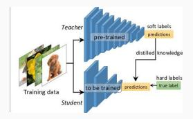
We construct a soft label, this is normally the final layer of the embedding from the larger model:
