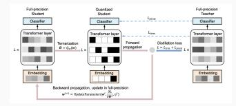
Activation loss, the second distillation loss: the loss between teacher model's attention scores from all attention heads in all layers and the student model's attention scores.
